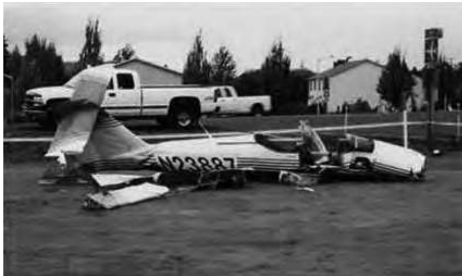
A flight instructor and his student were paralyzed when the plane they rented crashed following takeoff. The culprit was determined to be a malfunctioning carburetor that had not been maintained in over 10 years.
